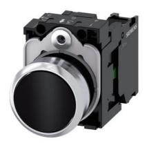
Pushbutton, 22 mm, round, metal, shiny, black, pushbutton, flat, momentary contact type, with holder, 1 NO, screw terminal, Z=20-unit packaging
