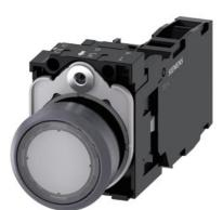
Illuminated pushbutton, 22 mm, round, plastic with metal front ring, clear, pushbutton, flat, momentary contact type, with holder, 1 NO+1 NC, LED module with integrated LED 230 V AC, screw terminal
