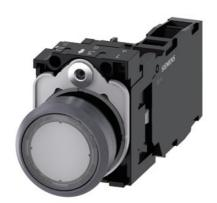
Illuminated pushbutton, 22 mm, round, plastic with metal front ring, clear, pushbutton, flat, momentary contact type, with holder, 1 NO+1 NC, LED module with integrated LED 230 V AC, screw terminal, with laser labeling, inscription or symbol Customer-specific selection with SIRIUS ACT configurator (CIN)
