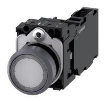
Illuminated pushbutton, 22 mm, round, plastic with metal front ring, clear, pushbutton, flat, momentary contact type, with holder, 1 NO+1 NC, LED module with integrated LED 230 V AC, screw terminal, with laser labeling, upper case and lower case, Always upper case at the beginning of the word
