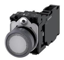
Illuminated pushbutton, 22 mm, round, plastic with metal front ring, clear, pushbutton, flat, momentary contact type, with holder, 1 NO+1 NC, LED module with integrated LED 230 V AC, screw terminal, with laser labeling, upper case
