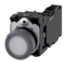
Illuminated pushbutton, 22 mm, round, plastic with metal front ring, clear, pushbutton, flat, momentary contact type, with holder, 1 NO+1 NC, LED module with integrated LED 230 V AC, screw terminal, Z=20-unit packaging
