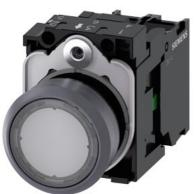
Illuminated pushbutton, 22 mm, round, plastic with metal front ring, clear, pushbutton, flat, momentary contact type, with holder, 1NO, LED module with integrated LED 230 V AC, screw terminal, with laser labeling, upper case and lower case, Always upper case at the beginning of the word
