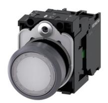
Illuminated pushbutton, 22 mm, round, plastic with metal front ring, white, pushbutton, flat, momentary contact type, with holder, 1NO, LED module with integrated LED 230 V AC, screw terminal, with laser labeling, lower case
