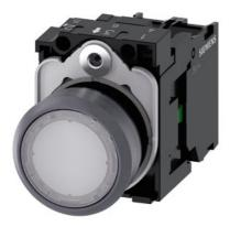
Illuminated pushbutton, 22 mm, round, plastic with metal front ring, white, pushbutton, flat, momentary contact type, with holder, 1NO, LED module with integrated LED 230 V AC, screw terminal, with laser labeling, upper case and lower case, always upper case at beginning of line
