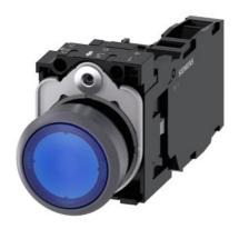
Illuminated pushbutton, 22 mm, round, plastic with metal front ring, blue, pushbutton, flat, momentary contact type, with holder, 1 NO+1 NC, LED module with integrated LED 230 V AC, screw terminal, with laser labeling, upper case and lower case, Always upper case at the beginning of the word
