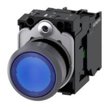
Illuminated pushbutton, 22 mm, round, plastic with metal front ring, blue, pushbutton, flat, momentary contact type, with holder, 1NO, LED module with integrated LED 230 V AC, screw terminal, with laser labeling, upper case and lower case, Always upper case at the beginning of the word
