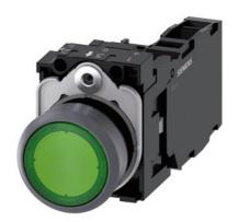
Illuminated pushbutton, 22 mm, round, plastic with metal front ring, green, pushbutton, flat, momentary contact type, with holder, 1 NO+1 NC, LED module with integrated LED 230 V AC, screw terminal, with laser labeling, lower case
