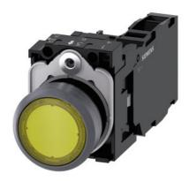
Illuminated pushbutton, 22 mm, round, plastic with metal front ring, yellow, pushbutton, flat, momentary contact type, with holder, 1 NO+1 NC, LED module with integrated LED 230 V AC, screw terminal, with laser labeling, upper case and lower case, Always upper case at the beginning of the word
