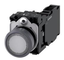
Illuminated pushbutton, 22 mm, round, plastic with metal front ring, clear, pushbutton, flat, momentary contact type, with holder, 1 NO+1 NC, LED module with integrated LED 110 V AC, screw terminal, with laser labeling, upper case and lower case, Always upper case at the beginning of the word
