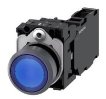
Illuminated pushbutton, 22 mm, round, plastic with metal front ring, blue, pushbutton, flat, momentary contact type, with holder, 1 NO+1 NC, LED module with integrated LED 110 V AC, screw terminal, with laser labeling, lower case
