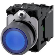
Illuminated pushbutton, 22 mm, round, plastic with metal front ring, blue, pushbutton, flat, momentary contact type, with holder, 1NO, LED module with integrated LED 110 V AC, screw terminal, with laser labeling, upper case and lower case, Always upper case at the beginning of the word
