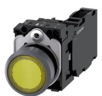
Illuminated pushbutton, 22 mm, round, plastic with metal front ring, yellow, pushbutton, flat, momentary contact type, with holder, 1 NO+1 NC, LED module with integrated LED 110 V AC, screw terminal, with laser labeling, upper case
