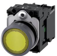
Illuminated pushbutton, 22 mm, round, plastic with metal front ring, yellow, pushbutton, flat, momentary contact type, with holder, 1NO, LED module with integrated LED 110 V AC, screw terminal, with laser labeling, upper case and lower case, Always upper case at the beginning of the word
