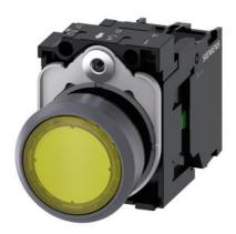
Illuminated pushbutton, 22 mm, round, plastic with metal front ring, yellow, pushbutton, flat, momentary contact type, with holder, 1NO, LED module with integrated LED 110 V AC, screw terminal, with laser labeling, upper case and lower case, always upper case at beginning of line
