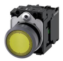
Illuminated pushbutton, 22 mm, round, plastic with metal front ring, yellow, pushbutton, flat, momentary contact type, with holder, 1NO, LED module with integrated LED 110 V AC, screw terminal, Z=20-unit packaging
