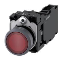
Illuminated pushbutton, 22 mm, round, plastic with metal front ring, red, pushbutton, flat, momentary contact type, with holder, 1 NO+1 NC, LED module with integrated LED 110 V AC, screw terminal, with laser labeling, symbol number according to, ISO 7000 or IEC 60417
