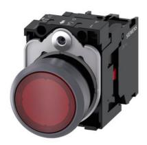
Illuminated pushbutton, 22 mm, round, plastic with metal front ring, red, pushbutton, flat, momentary contact type, with holder, 1NC, LED module with integrated LED 110 V AC, screw terminal, with laser labeling, upper case and lower case, always upper case at beginning of line
