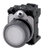
Indicator light, in illuminated pushbutton design, 22 mm, round, plastic with metal front ring, white, with holder, LED module, with integrated LED 24 V AC/DC, Spring-type terminal
