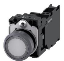
Illuminated pushbutton, 22 mm, round, plastic with metal front ring, clear, pushbutton, flat, momentary contact type, with holder, 1 NO+1 NC, LED module with integrated LED 24 V AC/DC, spring-type terminal, with laser labeling, inscription or symbol Customer-specific selection with SIRIUS ACT configurator (CIN)
