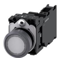
Illuminated pushbutton, 22 mm, round, plastic with metal front ring, clear, pushbutton, flat, momentary contact type, with holder, 1 NO+1 NC, LED module with integrated LED 24 V AC/DC, spring-type terminal, with laser labeling, upper case
