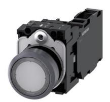
Illuminated pushbutton, 22 mm, round, plastic with metal front ring, clear, pushbutton, flat, momentary contact type, with holder, 1 NO+1 NC, LED module with integrated LED 24 V AC/DC, screw terminal, with laser labeling, upper case
