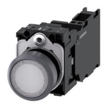
Illuminated pushbutton, 22 mm, round, plastic with metal front ring, white, pushbutton, flat, momentary contact type, with holder, 1 NO+1 NC, LED module with integrated LED 24 V AC/DC, spring-type terminal, with laser labeling, upper case
