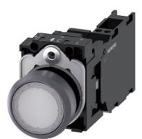
Illuminated pushbutton, 22 mm, round, plastic with metal front ring, white, pushbutton, flat, momentary contact type, with holder, 1 NO+1 NC, LED module with integrated LED 24 V AC/DC, spring-type terminal, Z=20-unit packaging
