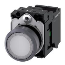
Illuminated pushbutton, 22 mm, round, plastic with metal front ring, white, pushbutton, flat, momentary contact type, with holder, 1NO, LED module with integrated LED 24 V AC/DC, spring-type terminal, with laser labeling, upper case and lower case, always upper case at beginning of line
