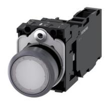
Illuminated pushbutton, 22 mm, round, plastic with metal front ring, white, pushbutton, flat, momentary contact type, with holder, 1 NO+1 NC, LED module with integrated LED 24 V AC/DC, screw terminal, with laser labeling, lower case
