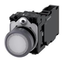
Illuminated pushbutton, 22 mm, round, plastic with metal front ring, white, pushbutton, flat, momentary contact type, with holder, 1 NO+1 NC, LED module with integrated LED 24 V AC/DC, screw terminal, with laser labeling, upper case and lower case, always upper case at beginning of line
