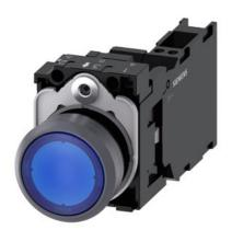
Illuminated pushbutton, 22 mm, round, plastic with metal front ring, blue, pushbutton, flat, momentary contact type, with holder, 1 NO+1 NC, LED module with integrated LED 24 V AC/DC, spring-type terminal, with laser labeling, symbol number according to, ISO 7000 or IEC 60417
