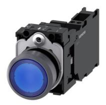
Illuminated pushbutton, 22 mm, round, plastic with metal front ring, blue, pushbutton, flat, momentary contact type, with holder, 1 NO+1 NC, LED module with integrated LED 24 V AC/DC, spring-type terminal, with laser labeling, upper case
