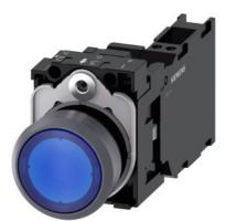
Illuminated pushbutton, 22 mm, round, plastic with metal front ring, blue, pushbutton, flat, momentary contact type, with holder, 1 NO+1 NC, LED module with integrated LED 24 V AC/DC, spring-type terminal, with laser labeling, upper case and lower case, always upper case at beginning of line
