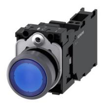
Illuminated pushbutton, 22 mm, round, plastic with metal front ring, blue, pushbutton, flat, momentary contact type, with holder, 1 NO+1 NC, LED module with integrated LED 24 V AC/DC, spring-type terminal, Z=20-unit packaging
