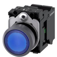
Illuminated pushbutton, 22 mm, round, plastic with metal front ring, blue, pushbutton, flat, momentary contact type, with holder, 1NO, LED module with integrated LED 24 V AC/DC, spring-type terminal, with laser labeling, lower case
