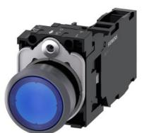
Illuminated pushbutton, 22 mm, round, plastic with metal front ring, blue, pushbutton, flat, momentary contact type, with holder, 1 NO+1 NC, LED module with integrated LED 24 V AC/DC, screw terminal, with laser labeling, upper case and lower case, Always upper case at the beginning of the word
