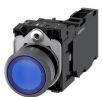
Illuminated pushbutton, 22 mm, round, plastic with metal front ring, blue, pushbutton, flat, momentary contact type, with holder, 1 NO+1 NC, LED module with integrated LED 24 V AC/DC, screw terminal, Z=20-unit packaging
