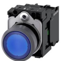
Illuminated pushbutton, 22 mm, round, plastic with metal front ring, blue, pushbutton, flat, momentary contact type, with holder, 1NO, LED module with integrated LED 24 V AC/DC, screw terminal, with laser labeling, inscription or symbol Customer-specific selection with SIRIUS ACT configurator (CIN)
