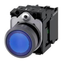
Illuminated pushbutton, 22 mm, round, plastic with metal front ring, blue, pushbutton, flat, momentary contact type, with holder, 1NO, LED module with integrated LED 24 V AC/DC, screw terminal, with laser labeling, symbol number according to, ISO 7000 or IEC 60417
