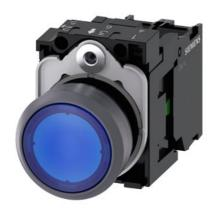
Illuminated pushbutton, 22 mm, round, plastic with metal front ring, blue, pushbutton, flat, momentary contact type, with holder, 1NO, LED module with integrated LED 24 V AC/DC, screw terminal, with laser labeling, lower case
