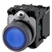
Illuminated pushbutton, 22 mm, round, plastic with metal front ring, blue, pushbutton, flat, momentary contact type, with holder, 1NO, LED module with integrated LED 24 V AC/DC, screw terminal, with laser labeling, upper case
