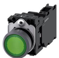
Illuminated pushbutton, 22 mm, round, plastic with metal front ring, green, pushbutton, flat, momentary contact type, with holder, 1 NO+1 NC, LED module with integrated LED 24 V AC/DC, spring-type terminal, with laser labeling, upper case and lower case, Always upper case at the beginning of the word
