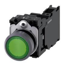
Illuminated pushbutton, 22 mm, round, plastic with metal front ring, green, pushbutton, flat, momentary contact type, with holder, 1 NO+1 NC, LED module with integrated LED 24 V AC/DC, spring-type terminal, with laser labeling, symbol number according to, ISO 7000 or IEC 60417
