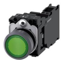
Illuminated pushbutton, 22 mm, round, plastic with metal front ring, green, pushbutton, flat, momentary contact type, with holder, 1 NO+1 NC, LED module with integrated LED 24 V AC/DC, spring-type terminal, with laser labeling, upper case
