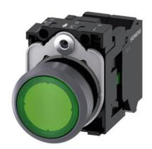
Illuminated pushbutton, 22 mm, round, plastic with metal front ring, green, pushbutton, flat, momentary contact type, with holder, 1NO, LED module with integrated LED 24 V AC/DC, spring-type terminal, with laser labeling, lower case
