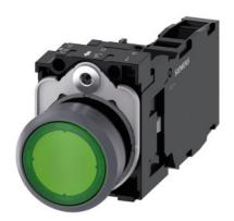
Illuminated pushbutton, 22 mm, round, plastic with metal front ring, green, pushbutton, flat, momentary contact type, with holder, 1 NO+1 NC, LED module with integrated LED 24 V AC/DC, screw terminal, with laser labeling, upper case and lower case, Always upper case at the beginning of the word
