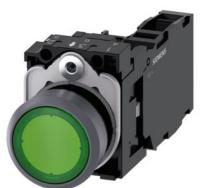
Illuminated pushbutton, 22 mm, round, plastic with metal front ring, green, pushbutton, flat, momentary contact type, with holder, 1 NO+1 NC, LED module with integrated LED 24 V AC/DC, screw terminal, with laser labeling, symbol number according to, ISO 7000 or IEC 60417
