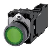
Illuminated pushbutton, 22 mm, round, plastic with metal front ring, green, pushbutton, flat, momentary contact type, with holder, 1 NO+1 NC, LED module with integrated LED 24 V AC/DC, screw terminal, with laser labeling, upper case
