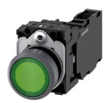
Illuminated pushbutton, 22 mm, round, plastic with metal front ring, green, pushbutton, flat, momentary contact type, with holder, 1 NO+1 NC, LED module with integrated LED 24 V AC/DC, screw terminal, with laser labeling, upper case and lower case, always upper case at beginning of line
